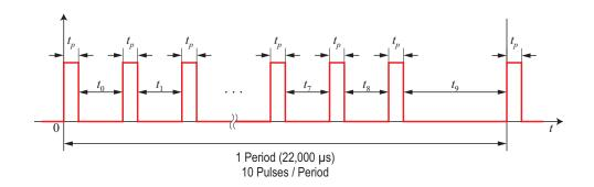
Figure 3.3: PPM waveform where  $t_p = 400 \,\mu s$ .
