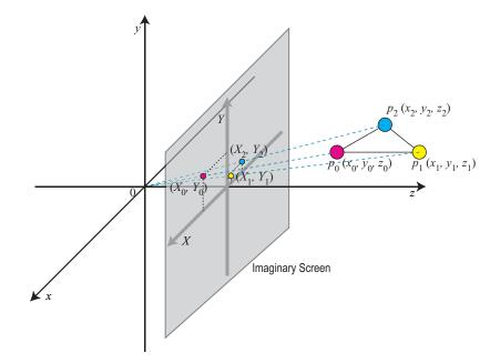
Figure 4.4: 2-D to 3-D conversion. Since the distance between each beacon's 3-D space is known, the three points on the imaginary screen can be uniquely converted into the 3-D coordinates with cross product verification.
