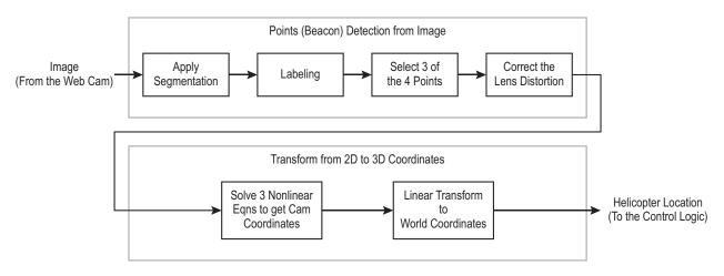
Figure 3.2: Overview of the Image Processor.
