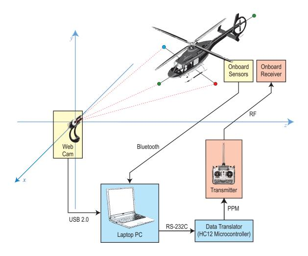
Figure 3.1: Overview of the system from the user's perspective.
