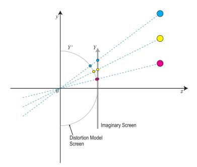
Figure 4.3: Lens distortion model. Using the geometry, the coordinates on the distorted screen can be mapped to the flat screen.
