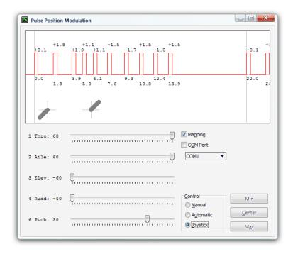
Figure 6.2: PPM signal generator.
