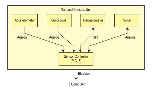
Figure 4.5: Overview of the Inertial Navigation System.
